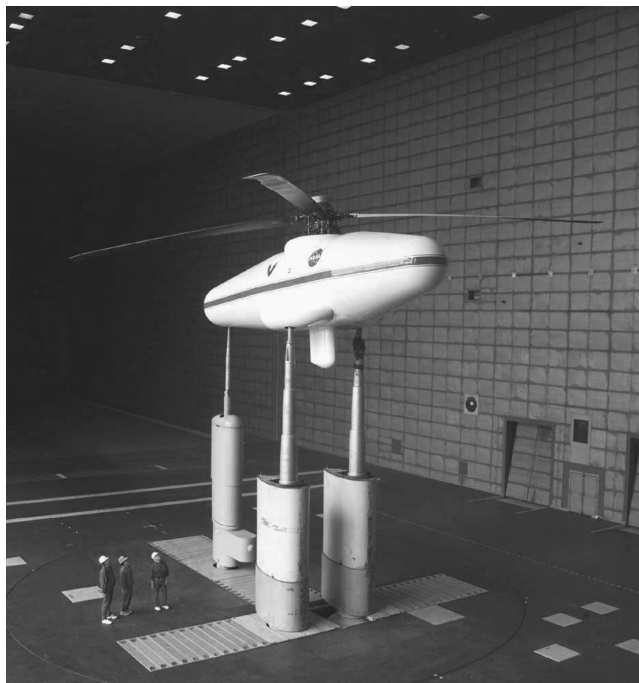
Fig. 2 Downstream view of the UH-60 rotor mounted on the LRTA in the 80- by 120-Foot Wind Tunnel at the NFAC at NASA Ames Research Center.
