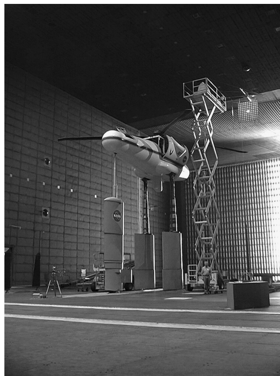
Fig. 6 Backlighted mapping target elevated to its position for rotor tests with its center at 12.8 m above test-section floor and in field of view of all three cameras.
